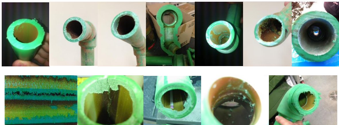
3) Copper ions harvested in PP-R HWRS pipes having a catalytic effect on oxidative stress cracking.
