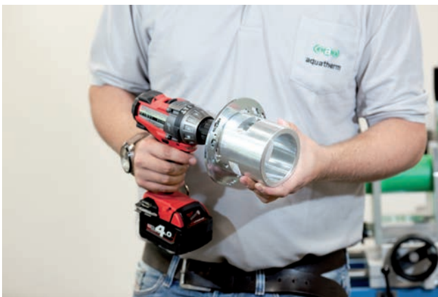
▲ Mechanical peeling process: Peeling tool with attachment plate
