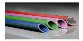
For the application in open air aquatherm offers composite **aquatherm green pipes** and **aquatherm blue pipes** with an UV-protective layer made from **black polyethylene** (PE with carbon black), which excludes damage caused by sunlight. This PE layer must be peeled off, prior to welding.
