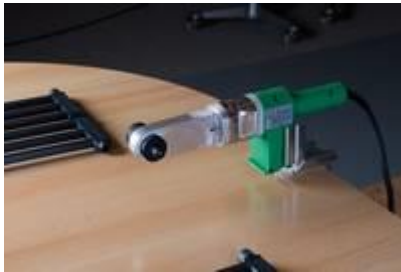
1) Mounted welding device and tools (16 mm) Control of temperature
