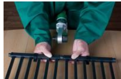
4) After the required warm-up time of 8 sec., remove the elements from the tools and immediately push together (welding depth 13 mm).
