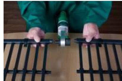
2) aquatherm black system is equipped with male/female connections for fusion in parallel.
