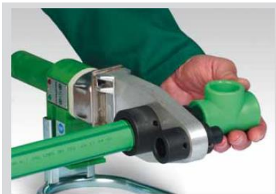
Heating-up of pipe and fitting
