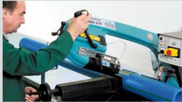
Before welding, pipes are cut into the required lengths
